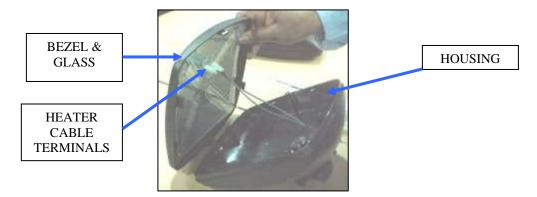
Remove the head clams screws and clamp (s). Make sure to save them for re-assembly.
