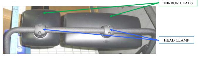
Remove the head clamp screws and the clamp(s). Make sure to save them for re-assembly. Remove the old mirror head(s) and replace them with the new mirror heads.
