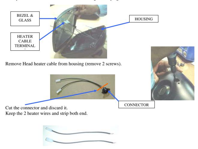
Assemble both black heater wires to the main heater cable.
