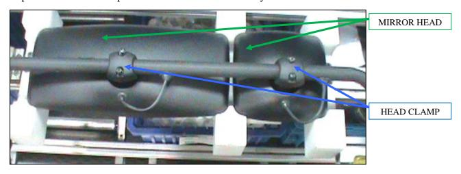
Unplug the 2 Heater cable connectors from both heads.
