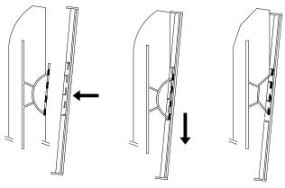
1. Actuate Socket Plate Down, Install Mirror Plate (Align Teeth)
