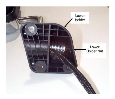
2. Remove the lower holder using a 13 mm socket.
