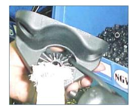
Slide the bolt through the tube connector.
